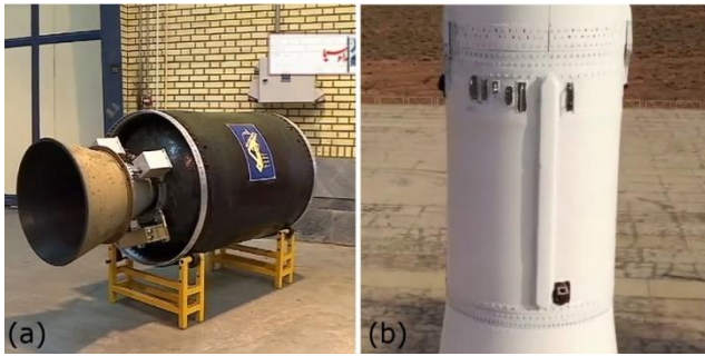
Figure 11: The Salman solid-propellant engine (a) and the Qased second stage (b). (Video stills from Iribmedia and Iranmedia.org)
