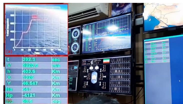
Figure 9: Screens from inside a ground station showing a graph of the total impulse as a function of time (inset a) and trajectory parameters at 392.3s after launch (inset b). (Original video still via Iranmedia.org)
