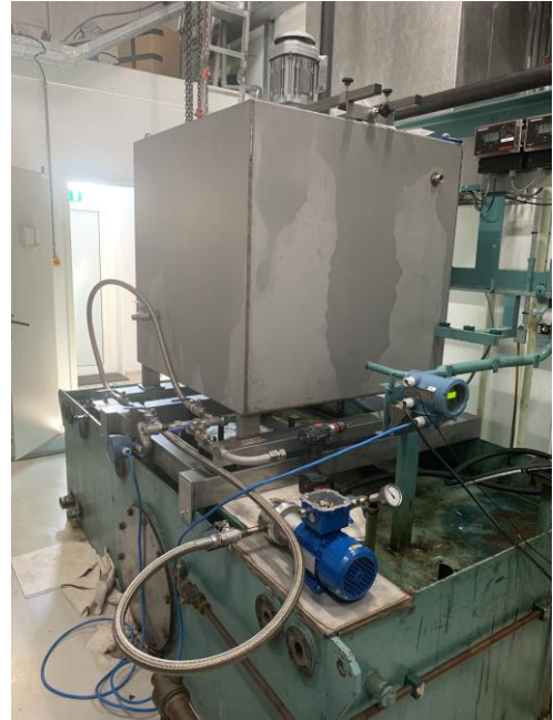
Figure 40: Modified fuel system: lay-out (left) and mix tank with stirring device mounted on the scale (right)
