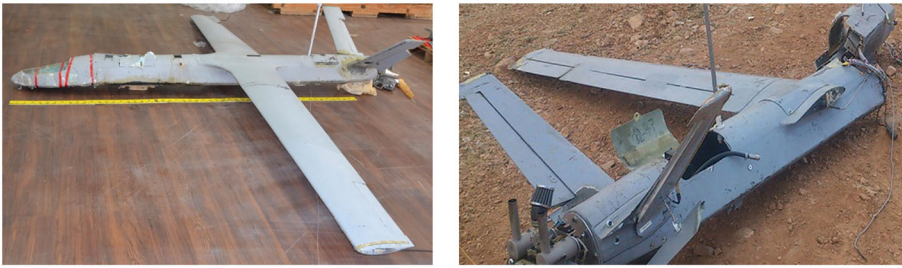
Figure 1. Reconstruction of Samad-2, length of 2.80 m (left); Samad-1 including details of the airfoil shape at the wing root (right). 15
